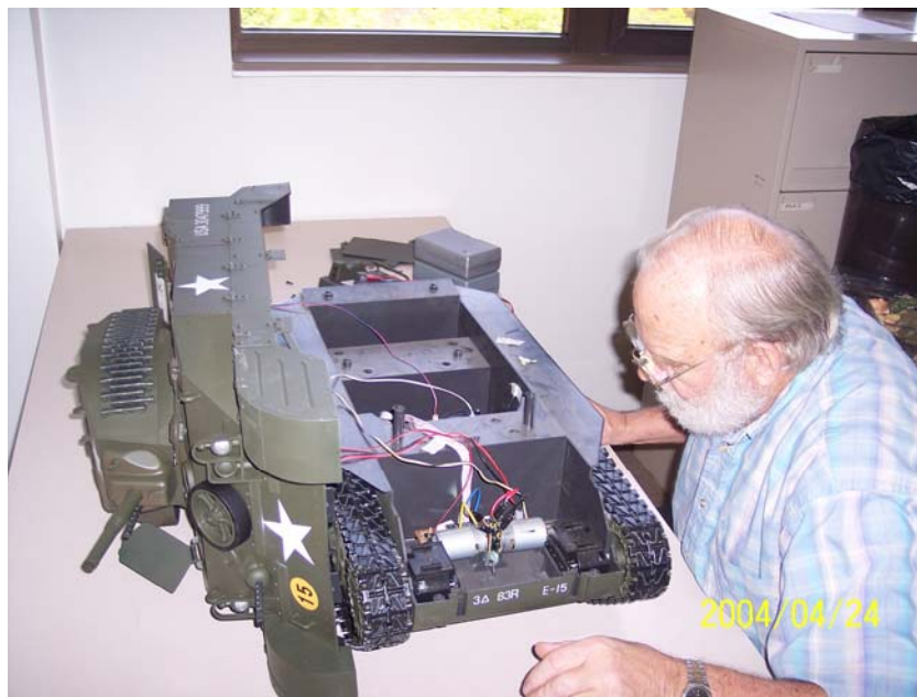
Fig. 5: Replacement of Internal RC Control Board with a WiFi-controlled Platform
