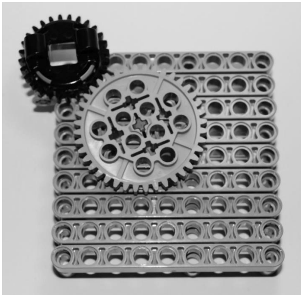
Figure 5. Non-Orthogonal Pairing of 28-Tooth Turntable and 40-Tooth Spur Gear
